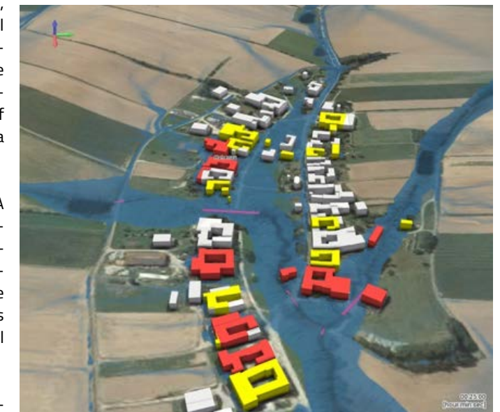
Figure 1: Example of pluvial flooding after 50mm of rainfall in 15 minutes; the building colour shows the maximum water depth: yellow = 50-100cm; red >100cm
