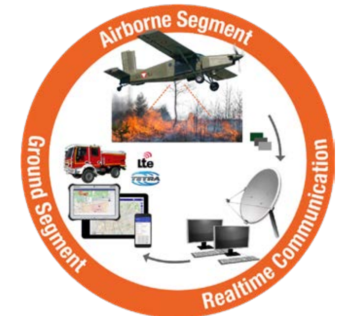
Figure 1: General concept of data acquisition, NRT communication and processing, data and resource management and information distribution to support time critical decision processes in forest fire situations
