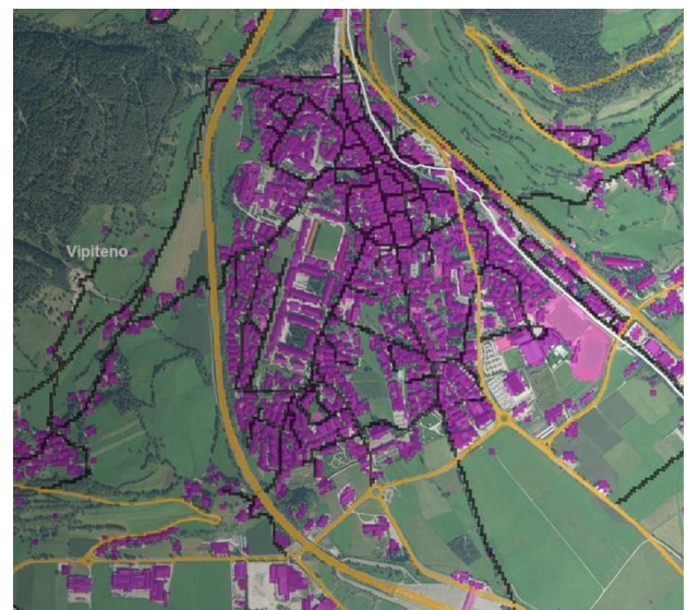
Figure 20: Rasterised asset information (buildings and road classes)
