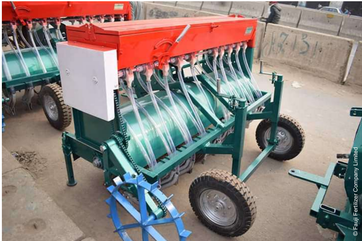
Photo 37. Locally manufactured Happy Seeder. The machine is compact, light-weight and tractor mounted. It consists of two separate units, a straw management unit and a sowing unit. The Happy Seeder can handle the paddy straw and do the sowing job without any tillage. It consists of straw cutting and chopping unit and a sowing drill combined in one machine. It sows the seeds of next crop in one operational pass of the field, while retaining the rice residue as surface mulch
