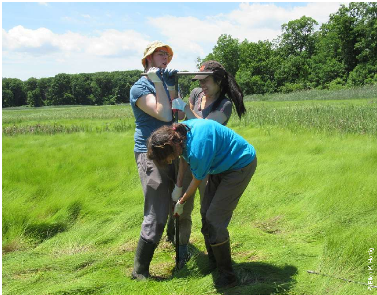
Photo 70. Members of Dr. Dorothy Peteet's New Core Laboratory extracting a peat core using the Dachnowski corer (a.k.a. Russian peat corer)
