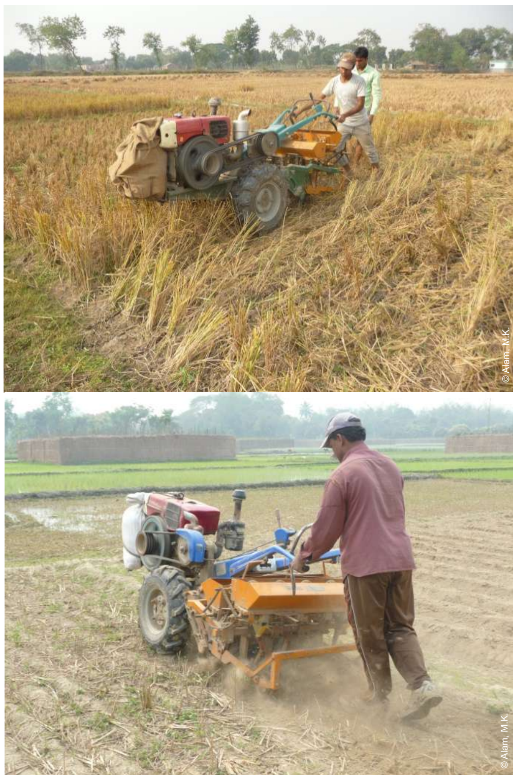
Photo 30. Two-wheel tractor with Versatile Multi-crop Planter (VMP), sowing through standing residue retained at higher rate at Digram, Rajshahi (top) and low rate (bottom) at Alipur, Durgapur, Rajshahi, Bangladesh
