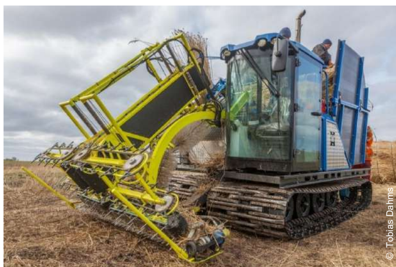
Photo 52. New designed harvester for cattail and common reed
