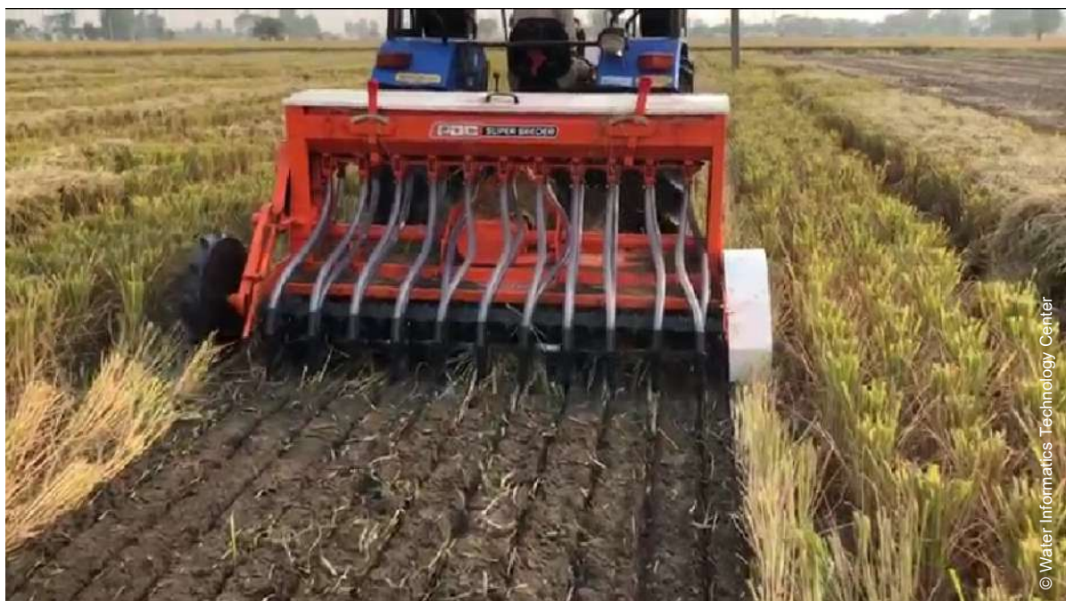
Photo 38. Farmer using “Super Seeder” to sow wheat immediately after mechanical harvest (using combine harvester) of paddy. At time of land preparation, about 26 liter per hectare less diesel is consumed on tillage operations. In addition, farmers can secure about 4 percent more grains compared to late sown wheat. Before introduction of mechanical harvest of the rice crop, residues were used as a fuel but now farmers seldom care about their collection from the field for fuel purpose
