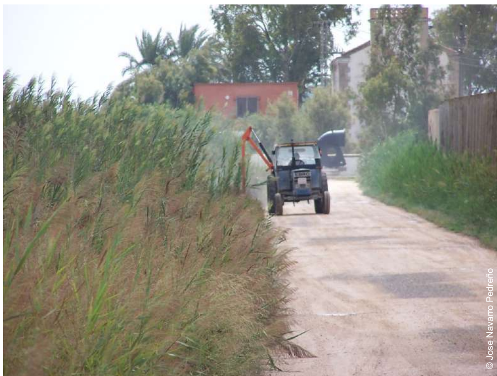
Photo 45. Machinery to cut the common reed. There is a similar machine that it is on a boat to cut from the drainage channels the plant
