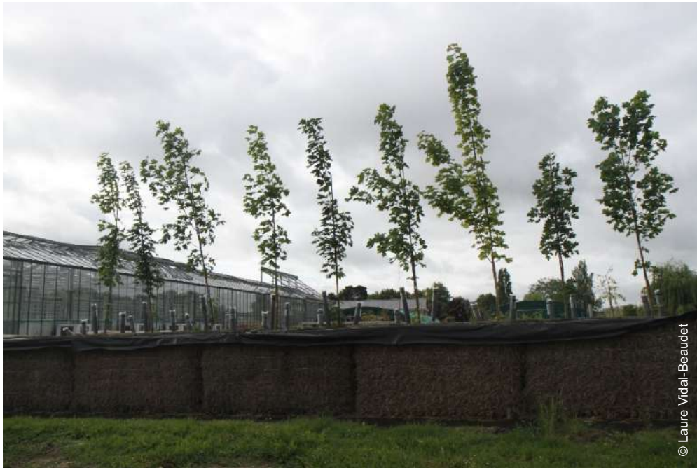
Photo 53. Experimental set up at AGROCAMPUS OUEST Angers (France), one year after planting. The 9 lysimeters are on the ground to facilitate their dismantling and sampling. Bales of straw were placed around them to insulate the lysimeters thermally and reproduce
