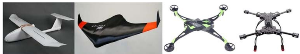
Fig. 1 Different airframes. From the left: polystyrene, plastic, aluminum, carbon fiber
