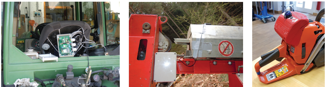
Figure 1. Three developed FDLs: On the left side the Tractor-FDL, in the center the Yarder-FDL, and on the right side the Chainsaw-FDL. The Tractor-FDL is the energy supplied by the electric circuit of the tractor, while the others foreseen the use of external batteries.
