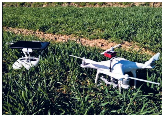
Figure 1. DJI Phantom 4 drone with a built-in Parrot Sequoia multispectral camera
