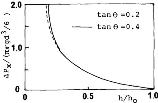
Fig.17 Pressure acting on the grain
