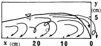
Fig.15 Trajectories of grains
