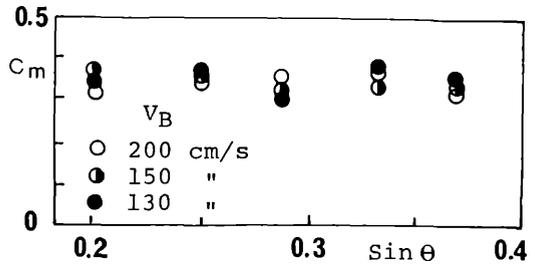
Fig.8 Mean concentration of debris flow
