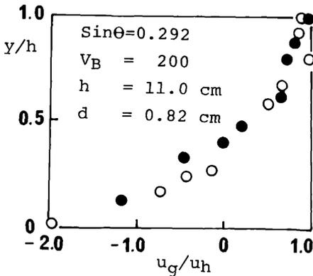
Fig.11 Velocity distribution of debris flow in a moving co-ordinate system
