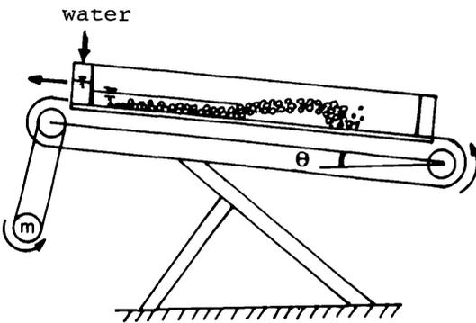
Fig.2 Experimental apparatus
