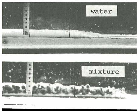
Fig.3 Shapes of bore
