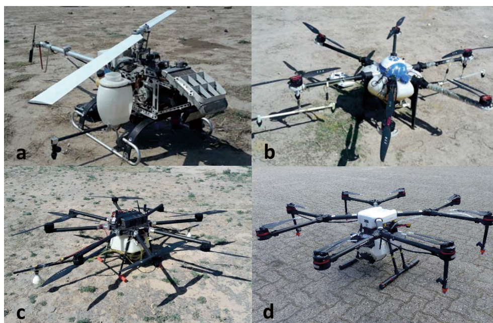
Fig. 1. UAASs involved in the study (a – 1 rotor, b – 6 rotor, c – 8 rotor (TTA) and d – 8 rotor (DJI)
